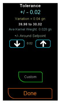
**<u>Line 1</u>**: Selected tolerance configuration. Blue indicates ± tolerance around the setpoint; Green indicates custom settings.
