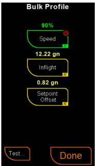
**Speed**: Defines the rotation speed from 1% to 100%. The default is 90%, but this may not suit all powders. Powders that flow poorly may clump or tumble inside the tube; reducing speed often improves consistency. A stable output allows the system to predict inflight powder more accurately, helping the bulk instrument stop closer to the target weight. See Bulk Test for more details. To disable the Bulk instrument, press and hold the Speed button.
