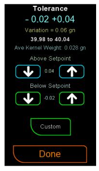
Custom Settings – Allow separate tolerance values below and above the setpoint.
