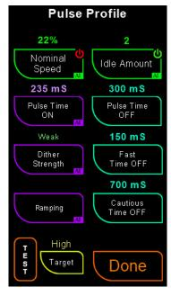
\* Idle Amount: When the tube starts there is considerable inertia involved before the kernels respond to the vibration and begin moving. The pulse idle amount is set in units, which can be a value between Off or 1 to 100, generally a value of 5 is considered high.
