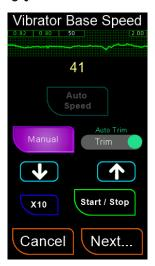
Alternatively, you can use the **Manual** setting to adjust the speed until the scale increments roughly once per second. Once this rate is achieved, stop the motor and reduce the speed by 4 units to optimize the control system's range.
