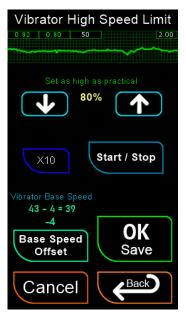
On the **Vibrator High Speed screen**, the base speed is shown along with the applied offset. To change the offset, press the **Base Speed Offset** button and enter a value between –20 and 0. If a positive number is entered, the system will automatically convert it to negative. If the value is out of range, the default offset will be used.
