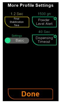
\* <u>Final Stabilization Time</u>: Final Stabilization Time – This parameter, measured in seconds, defines the delay after a charge completes. It gives the scale time to stabilize before determining whether the charge needs more powder, is within tolerance, or should be rejected due to overshoot.
