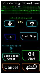
The job of the vibrator high speed limit is exactly what is says: to limit the speed that any of the vibrator instruments can go. This setting has a range between 1 to 100%.
