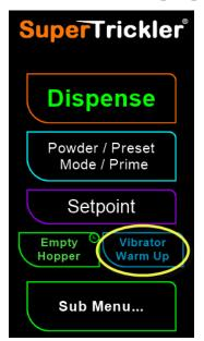
**Before Filling with Powder,** It is recommended to use this option to run the vibrator without powder in order to warm up the rubber mount. This can lead to more stable operation. The warm-up process can be started and run on a background timer while other tasks are being carried out.
