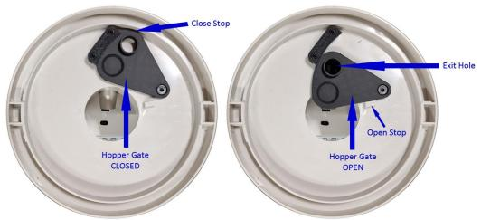
The SuperTrickler will not seat into position on the scale if the hopper gate is not fully closed, to prevent accidental spillage of powder.
