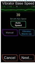
The adjustment range available is between 1 and 255 units. This value represents 1% speed for all the vibrating instruments.
