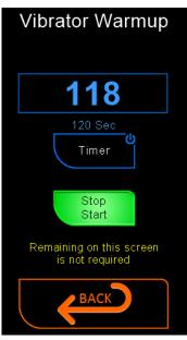
Use the green button to start or stop the operation. If a timer is set, the vibrator will run for the specified duration—remaining on the screen is not required. To stop the vibration before the timer expires, simply touch the green Start/Stop button again. Without the timer running existing the screen will stop the vibrator.
