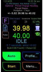
be un-primed (we will learn how to do this later), so you may find that after about 5 seconds, a **DISCARD** error will appear with a "No Weight Detected" message. Just press **Start** again and repeat until the powder begins to flow from the bulk tube.
