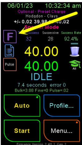
The statistics hold to reset button has now been replaced with a single touch 'F' function key. Pressing this will bring a function page to allow you to select what function or functions you would like to carry out.
