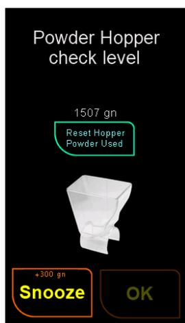
When the alarm pops up, you can select Snooze, this will add 300 grains to the target threshold. The alert will disappear and normal operations will continue.
