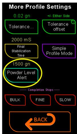
When a charge is successful, the powder used is added to the register. When the register reaches the value set by the profiles Powder Level Alert a warning will be issued, as the cup is removed from the pan.
