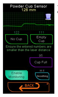
To calibrate the Cup Full, turn the standard SuperTrickler® cup upside down on the platen and use the base as the warning level.
