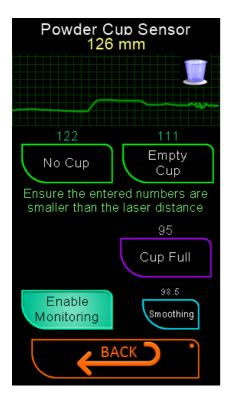
To calibrate the Cup Full, turn the standard SuperTrickler<sup>®</sup> cup upside down on the platen and use the base as the warning level.
