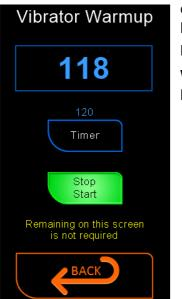
optional timer can be set (and retained) in seconds. This option allows you to leave the warm-up screen and proceed with other tasks such as choosing a powder or profile, etc.
