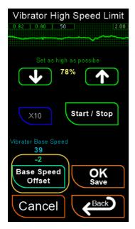
From this screen, the Vibrator Base Speed is shown along with the offset value. The base speed is displayed with the offset value applied. In the event you choose to change this value, pressing the Base Speed Offset button will enable a new value between -20 to 0 to be applied. If you fail to make the value a negative number, the system will convert it automatically. An out-of-range value will result in the default offset being applied.
