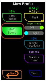
to around the one or two increments per second. Turning if off will use the fixed speed set by Slow Speed value and turning it on will use the initial slow speed setting however will change this value in order to keep the flow withing the operational range.
