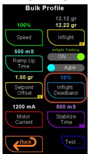
affect the pressure and consequently the powder flow to the tubes. However, with continuous changes in Bulk, Fine, and possibly Slow inflight tracking, these adjustments can counteract each other, adversely impacting overall performance.
