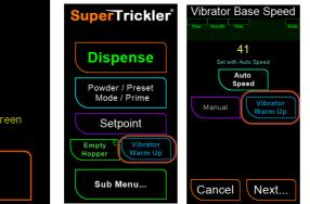
There are two access points to the warmup screen, the Main Menu or the Vibrator Base Speed screen.
