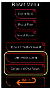
The top three small buttons will reset the respective instruments, and the three larger buttons will reset the profile (all instruments) in a distinctive way.
